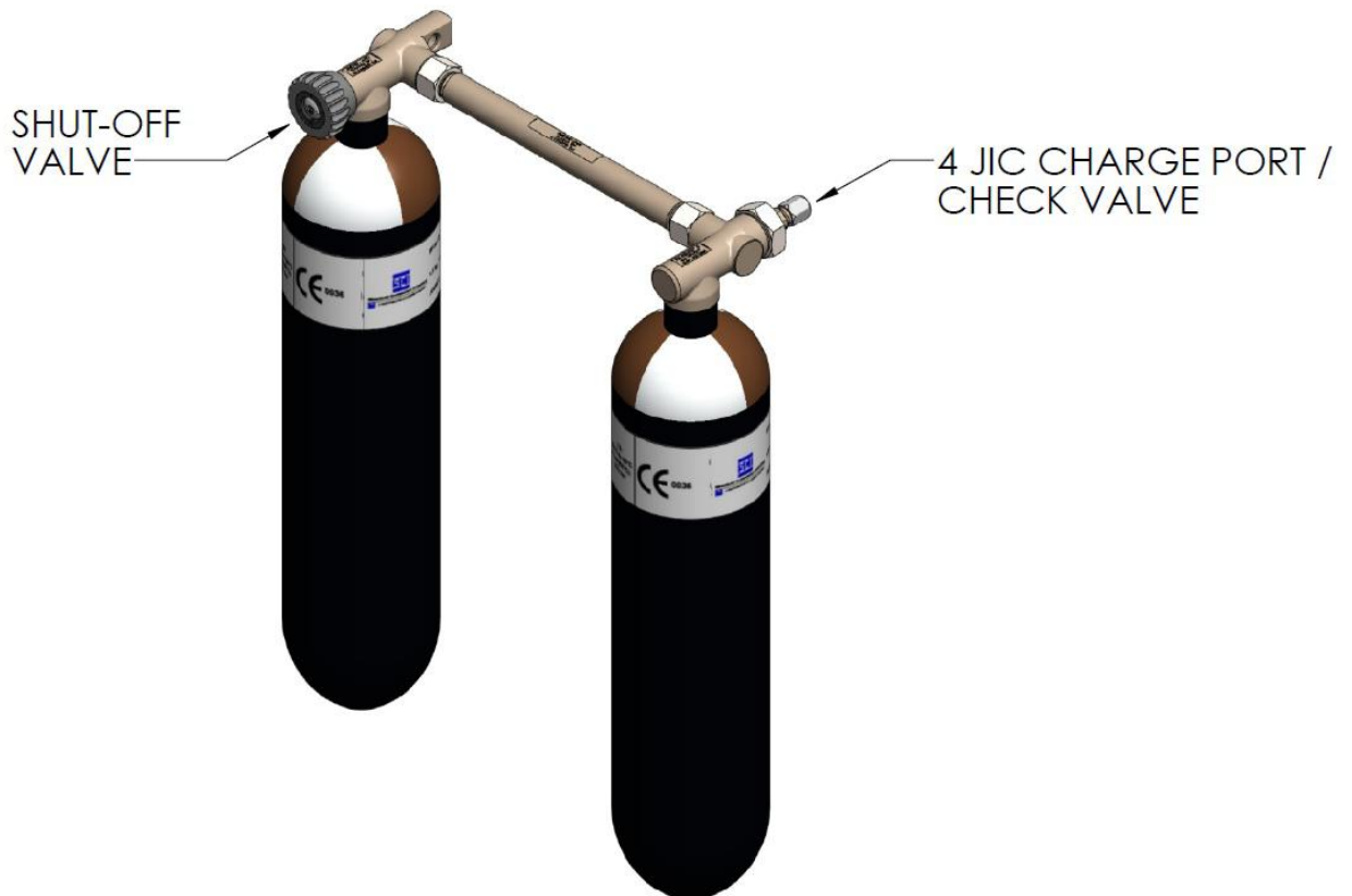
Figure 55 High Pressure Supply System
