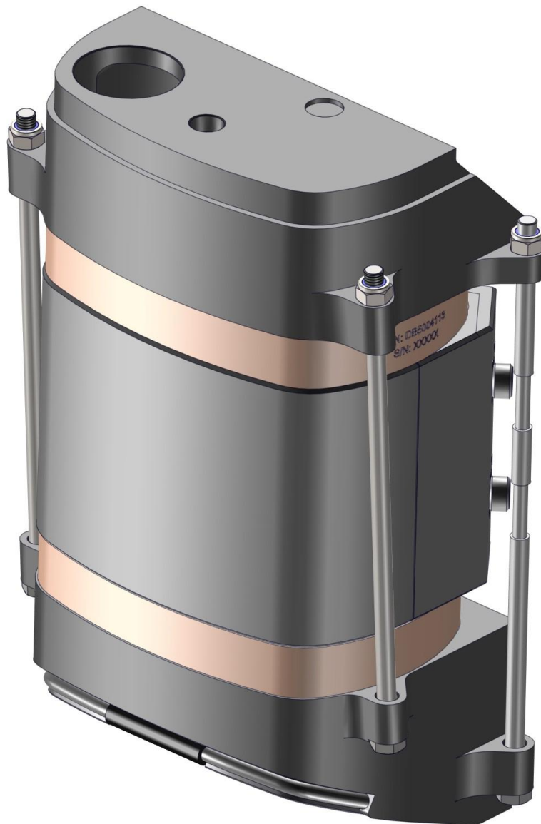
Figure 27 Revised Hot Water Housing
