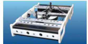
AX ring removal skid
