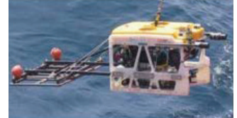
Survey skid with TSS pipe tracker
