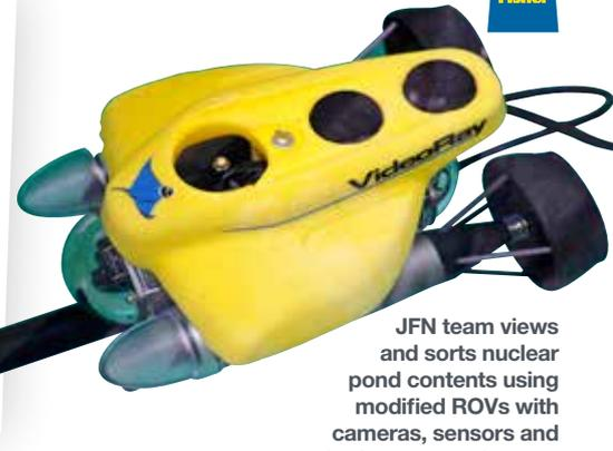
JFN team views and sorts nuclear pond contents using modified ROVs with cameras, sensors and robotic arm attachments
