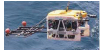
Survey skid with TSS pipe tracker
