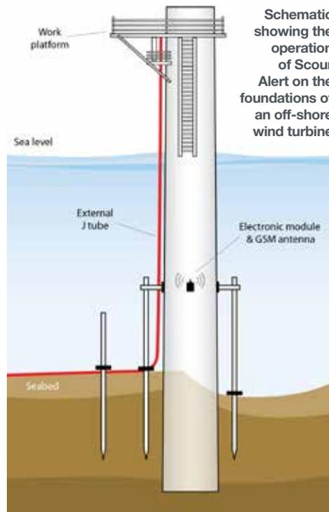
**Schematic showing the operation of ScourAlert on the foundations of an off-shore wind turbine**
