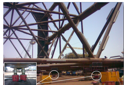
New type 7510 load cells being used to weigh large structure
